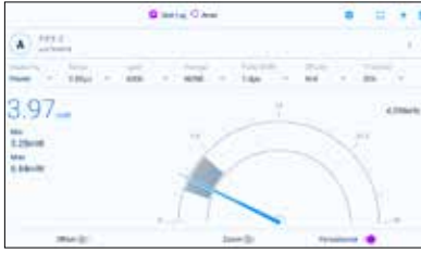
Analog needle display of power Persistence and min/max tracking.
