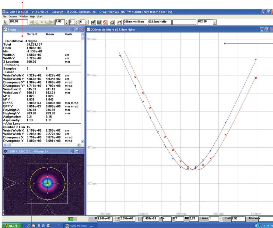
This window presents measurements of beam width vs. position for a given run. After measuring a few points, the software extrapolates a curve fit. The Xs and Ys represent individual measurement points. The solid lines present the best fit hyperbola of the beam propagation equation to the measured points. The M<sup>2</sup> and other laser parameters are computed from the best fit hyperbola since it provides a smoothing of the data points.
