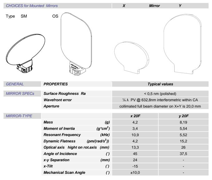
The Dynamic Flatness is a normalized measure given as the max. deformation (PV) of the mirror surface at a angle acceleration rate of 1 rad/s<sup>2</sup> Technical Datasheet 6020.10
