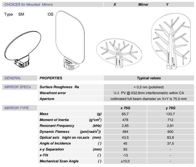
The Dynamic Flatness is a normalized measure given as the max. deformation (PV) of the mirror surface at a angle acceleration rate of 1 rad/s<sup>2</sup>
